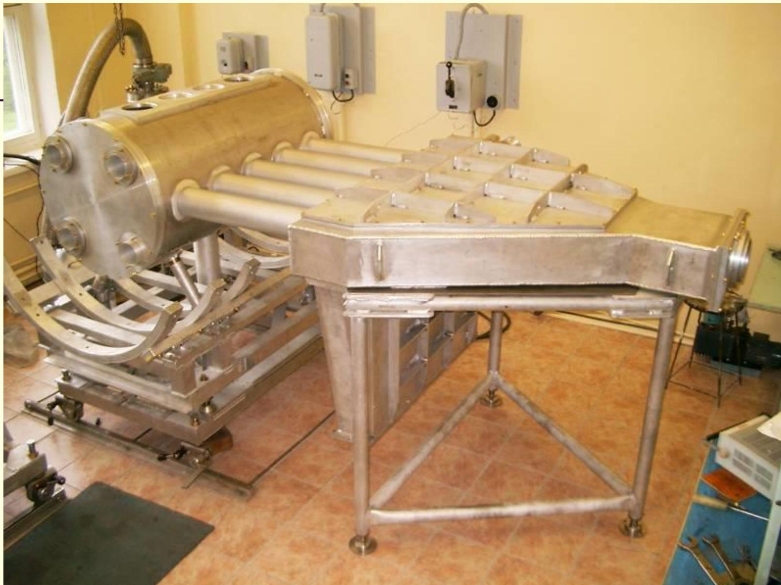
Housing of neutron guide system and vacuum chamber
