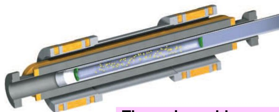
The trapping region is filled with superfluid  $^4\text{He}$ , which is used to load neutrons into the trap and as a scintillator to detect their decay. Neutrons have a lifetime in the trap of
